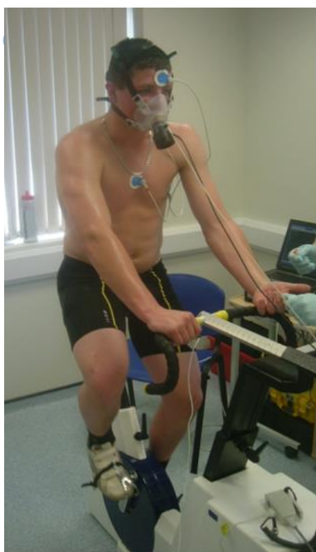
Figure 3 Experimental set-up of cardiopulmonary exercise test using a bioelectrical impedance cardiography system in people with long COVID (Source: Author)
