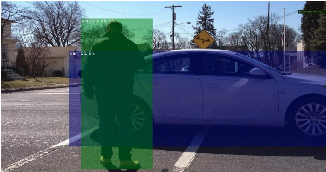
Figure 8: Test for object detection model, detected pedestrian
